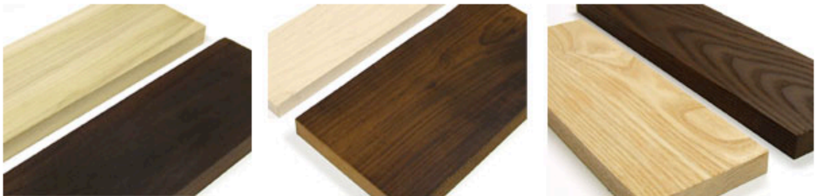
FROM LEFT: Bingaman Lumber photos show the color transformation as unfinished poplar, maple and pine darken during the thermal treatment process.
