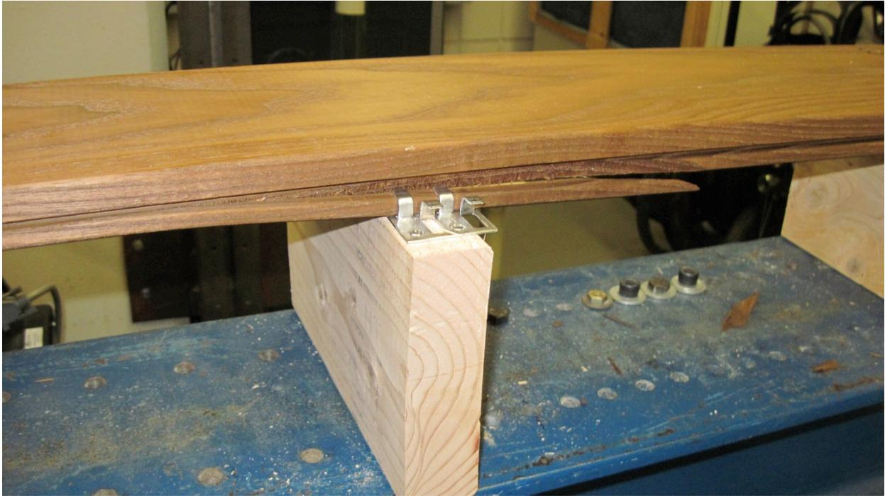
Figure 3.--Typical failure of lower tongue when decking installed with clips.
