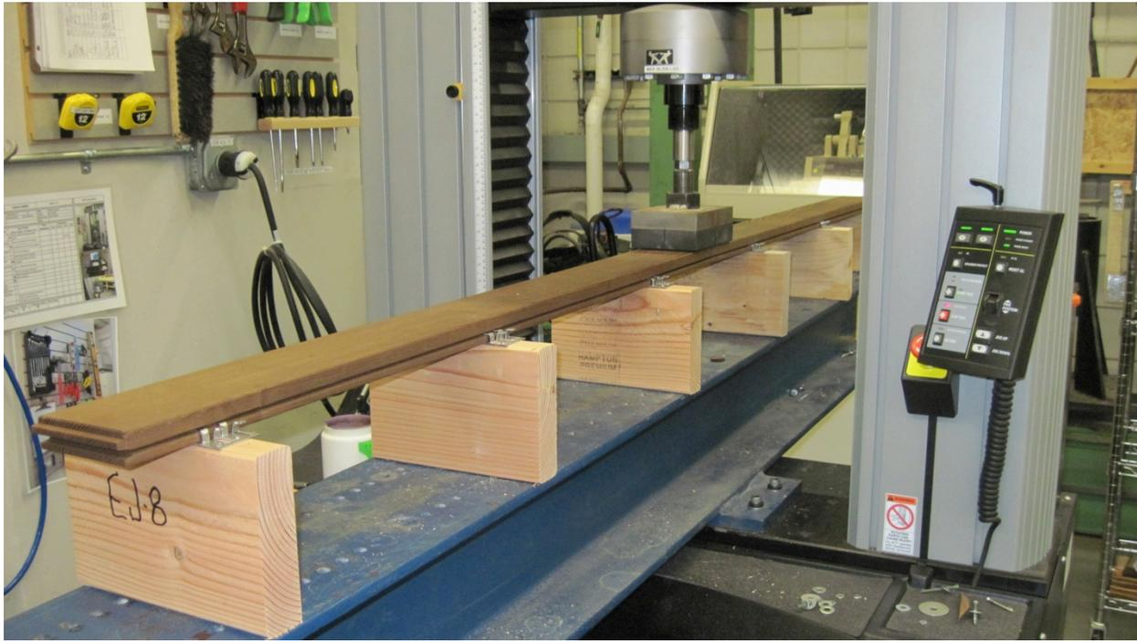
Figure 2.--Test setup showing decking spaced 16 in on-center with a 4- by 6-in. load surface above the end-joint. This sample was attached with clips attached to the joist edge and the decking groove.
