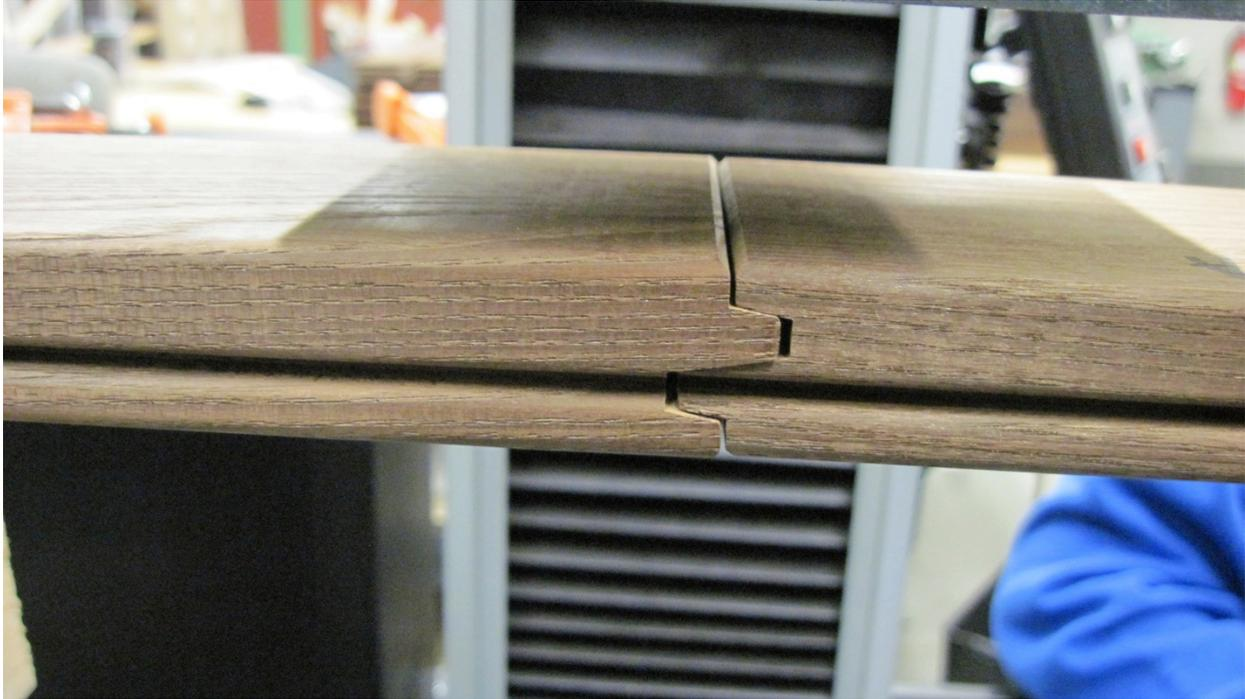
Figure 1.--End-joint tested to evaluate bending characteristics.
