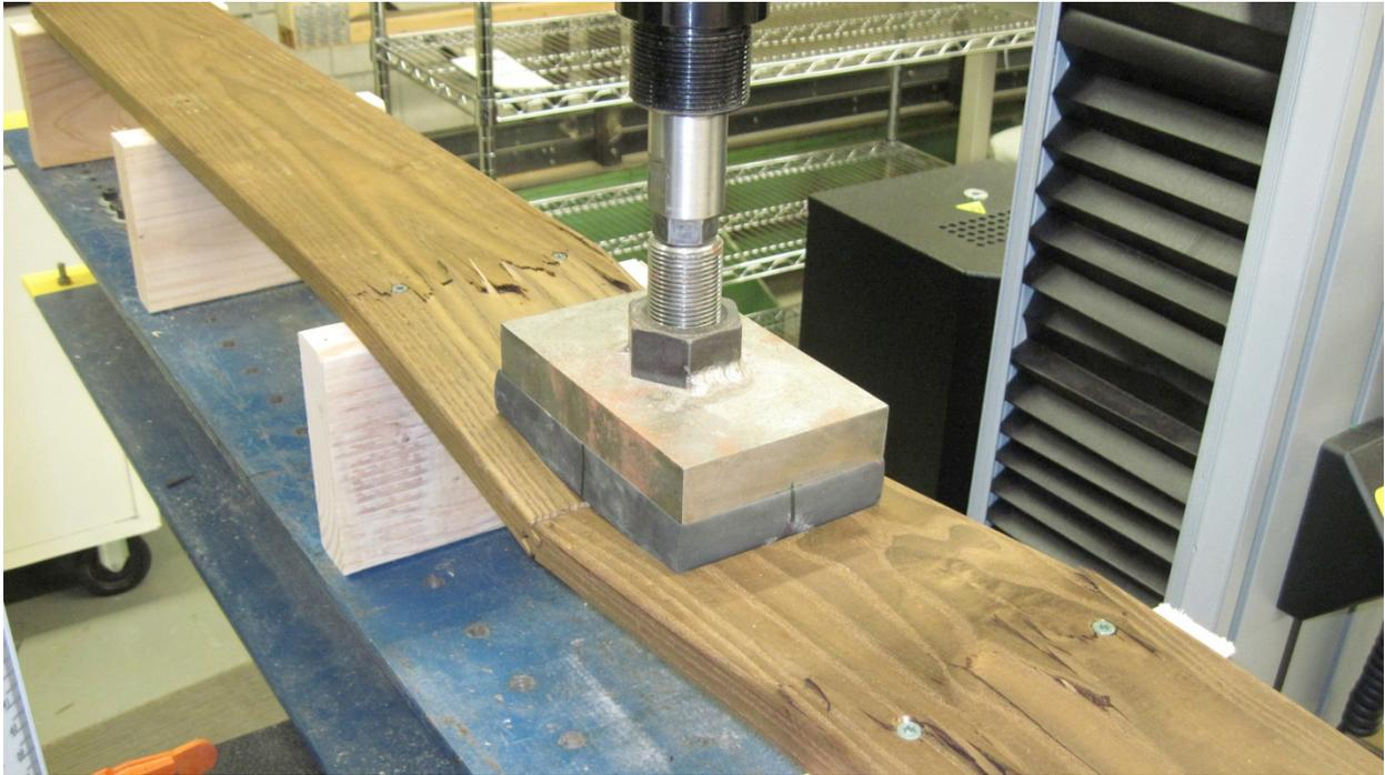
Figure 5.--Typical lumber showing failure mode. This sample was face-screwed to the joist edge.
